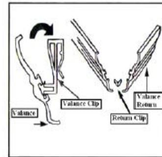
For an inside mount installation, insert the valance clips into the valance groove located on the backside of the valance. Afterwards, make sure the valance clip is securely fastened to the headrail before using your blind.
