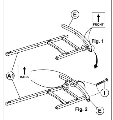
Attached each rocker (E) to right and left side frame (A1 & A2) as picture shown, connecting front of rocker to front legs first then the back of rockers. Secure connections with 1 3/4" Bolts (I).
