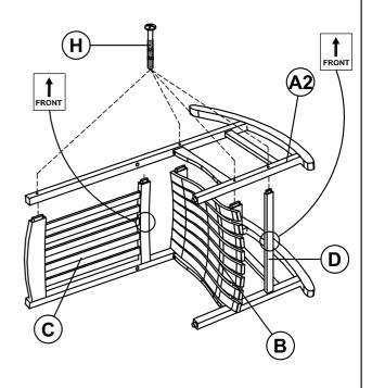
Install Seat (B), back support (C), and Apron (D) into corresponding holes of right side frame (A1). Attach the left side frame (A2) onto seat (B), back support (C), and apron (D). Secure left side frame (A2) using 1 1/4" bolts (H), as shown.
