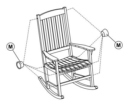
Make sure all parts are connected and tighten all bolts and screws completely using screwdriver. Tap in the wooden caps (M) to cover bolts head using rubber mallet.
