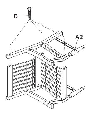
Attach the left side frame (A2) onto the pre-assembled and secure using 1 1/2" bolts (D).
