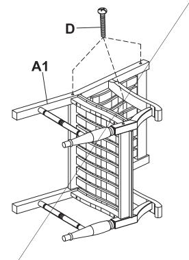
Turn the chair onto the other side and repeat step 2 to fasten the right side frame (A1).
