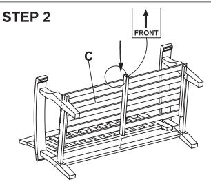
Put the seat (C) into predrilled holes of back apron as shown.
