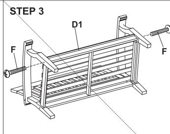
Next, attach the front apron (D1) into right and left side frames (A1 & A2).
