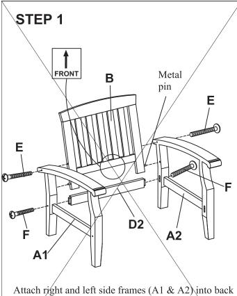
Attach right and left side frames (A1 & A2) into back support (B) and back apron (D2). Secure using 3 1/2" bolts (E) into back support and 2" bolts (F) into back apron as shown.
