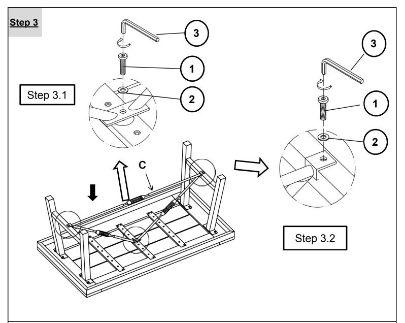
Attach the Turnbuckle frame (C) into assembled frame as shown in picture above.
