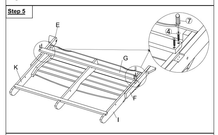
Position Front Support (G) onto the tract of Short Legs (E), (F) using 4 Screws (4) and Screwdriver (7).
