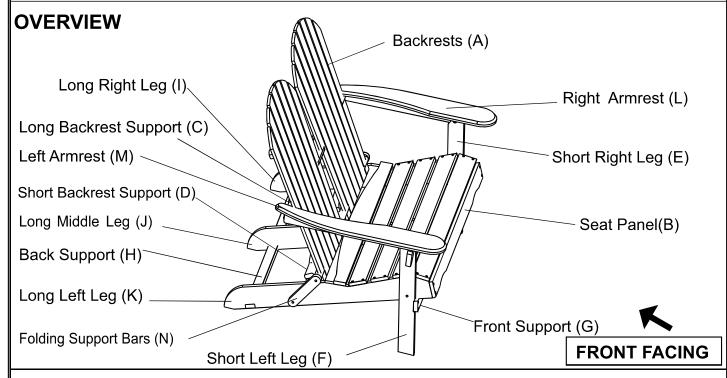
This LoveSeat has multiple parts and may require up to 30 minutes to assemble. To give you an overview of the LoveSeat parts, the above picture is to help you put the various parts into perspective. Please read through the instructions below to familiarise yourself with the parts and steps before assembly.
