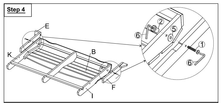
Attach Short Left Leg (E) and Short Right Leg (F) onto Long Left Leg (K) and Long Right Leg (I) using 2 Bolt (1), Plastic Washer (5) and Sleeve Nut (2) with Allen Wrench (6).
