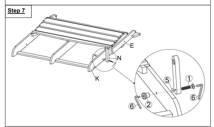
Reverse Seat panel in Step 5 in the position as picture above Attach Folding Support Bars (N) to Long Left Leg (K) using Bolt (1), Plastic Washer (5), Sleeve Nut (2) and Allen Wrench (6).
