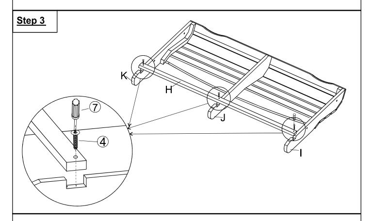
Position Back Support (H) on to the tract of Long Legs (I), (J), (K) using 3 Screws(4) and Screwdriver (7).
