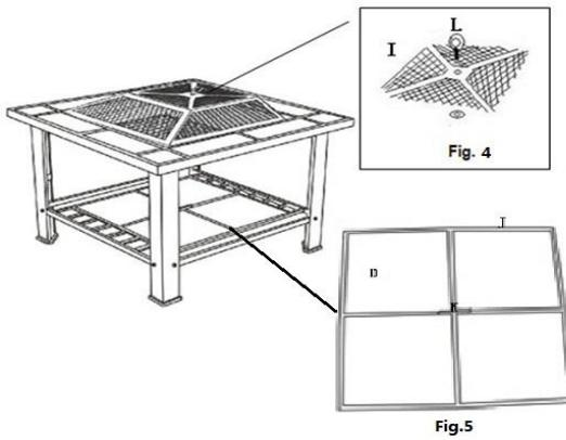
**Step 5)** For Table use: fix Handle (K) to Lid Frame (J), put Big Square Ceramic Tile (D) onto Lid Frame (J). Put assembled table lid into tabletop frame.
