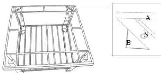
**Step 3)** Tighten all the bolts accordingly with the provided Allen Wrench (Q) until all pieces fit together securely after Step 2. Place Small Square Ceramic Tile (E) and Rectangular Ceramic Tile (F) onto the assembled frame, then put Square Bowl (G) and Log Grate (H) into the assembled frame.
