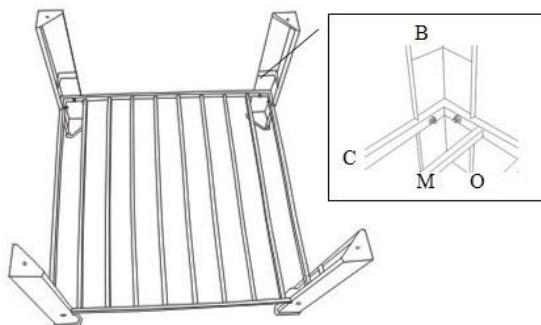
**Step 2)** Attach Top Frame (A) to Leg (B) by using Bolt (N). Tighten by hand and do not fully tighten all bolts.
