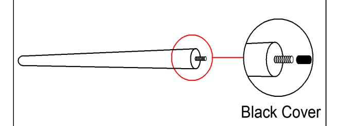
Open the carton and place all parts onto a clean, non-marring surface. Remove the Black Cover on the threaded stem of the Legs(B).
