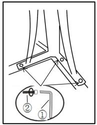
Attach two Front Legs(C1) to the Basket Seat(A) using Bolts with Washers(②) with Allen Key(①) as shown in the picture above.
