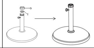
For the Umbrela Pole with diameter as 38mm, use Dia. 38mm Adapter (H) & Dia. 48mm Adapter (I) added together, insert the Dia. 48mm Adapter (I) into the Support Pole (E) first, and then put the Dia. 38mm Adapter (H) onto the Dia. 48mm Adapter(I), Turn the Cap(G) onto the Support Pole(F) to hold the
