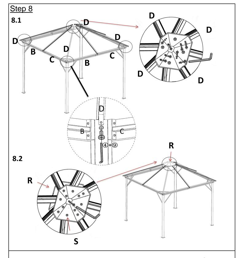
**8.1)** Attach Long Corner Roof Bars(D) to Inside Roof Connector(S) using Bolts(4) and Washers(9) with Allen Key(7).
