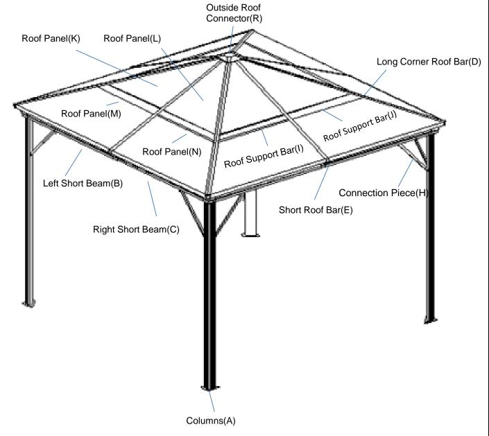
This Gazebo has multiple parts and may require up to 3 to 4 hours to assemble. To give you an overview of the Gazebo parts, the above picture is to help you put the various parts into perspective. Please read through the instructions below to familiarise yourself with the parts and steps before assembly.
