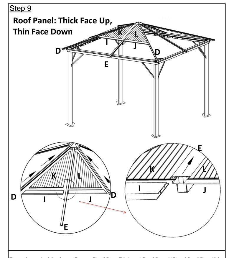
From the end of the Long Corner Roof Bars(D), insert Roof Panel(K) and Roof Panel(L) into the Roof Bar's upper tracks as pictured above.
