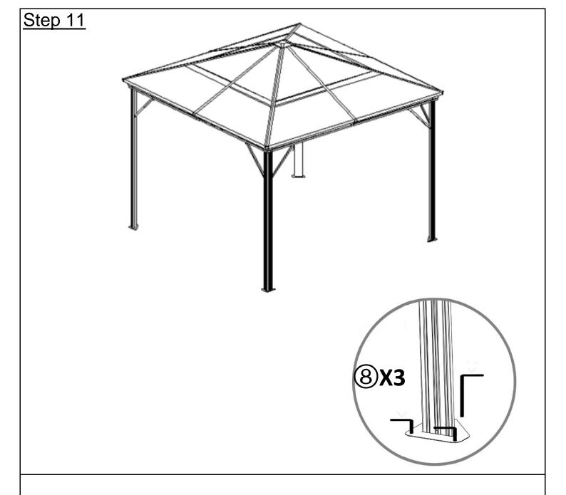
Affix the Gazebo to the ground by inserting the Stakes(③) through the Bases(T). Your Gazebo is ready for use.
