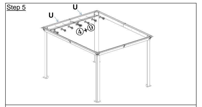
Attach Tracks(U) to the inside of Left Short Beams(B) and Right Short Beams(C) using Bolts(4) and Washers(9) with Allen Key(7).
