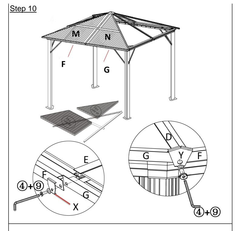
Insert the Roof Panel(M) and Roof Panel(N) into the Roof Bar's bottom tracks as pictured above.
