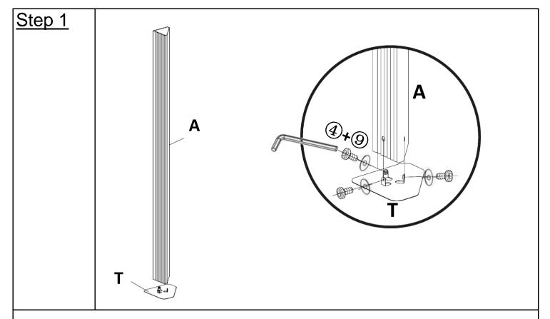
Attach Columns(A) onto Bases(T) using Bolts(4) and Washers(9) with Allen Key(7). **Do NOT fully tighten the bolts.**
