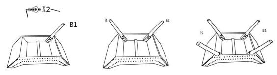
Install the legs on the leg position located on the underside of the Bench.
