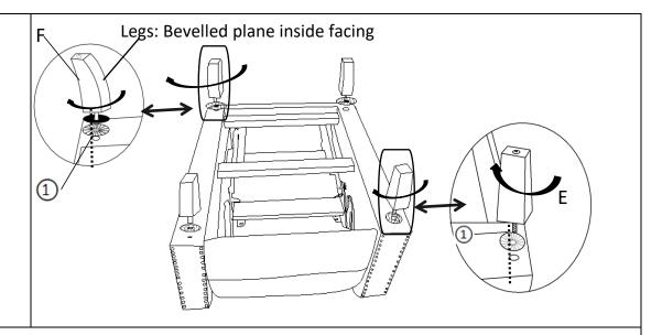
Install the Front Leg(E) and Hind Leg (F) at the bottom of the Chair by placing one Plastic Gasket(①) on the threaded stem.
