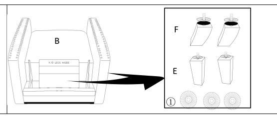
Place the Chair Base with Footrest(B) facedown on a clean, non-marring surface. Open the non-woven bag and take out the Front Leg with 1 Plastic Gasket(E), Hind Leg with 1 Silicone Gasket and 1 Plastic Gasket(F) and Plastic Gaskets(①).
