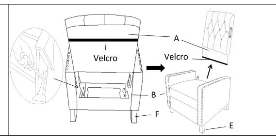
Disassembly Note:open the flap on the Chair Backrest(A),use a screwdriver(Don't use fingers) pressing outward on the metal ear on the preattached Metal Bracket on one side of the Chair Base(B),with assistance of you adult partner to keep the Chair Base(B) in place,pull out the Chair Backrest(A) upward at the same time,repeat the same step for another side. Then the Chair Backrest(A) can be taken out.
