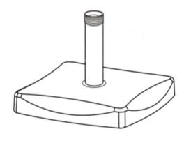
Screw in the Support Pole (B) onto the base.
