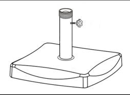
Screw the Adjustable Screw (C) into the Support Pole(B).
