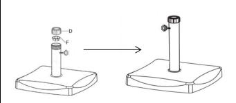
For the Umbrela Pole with diameter as 38mm, use Dia. 38mm Adapter (E) & Dia. 48mm Adapter (F) added together, insert the Dia. 48mm Adapter (F) into the Support Pole (B) first, and then put the Dia. 38mm Adapter (E) onto the Dia. 48mm Adapter(F), Turn the Cap(D) onto the Support Pole(B) to hold the Adapters in place.
