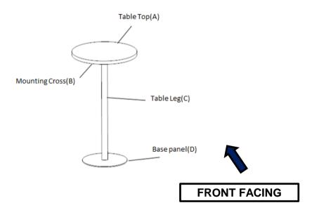
This Table has multiple parts and may require up to 15 minutes to assemble. To give you an overview of the Table parts, the above picture is to help you put the various parts into perspective. Please read through the instructions below to familiarise yourself with the parts and steps before assembly.
