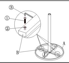
Attach the Table Top(A) to the Mounting Cross(B) and Table Leg(C) using Bolt(1) &Washer(2) with Allen Key(3) as shown in Picture.
