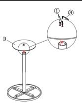
Attach the Base panel (D) to the Table Leg(C) using Bolt(1) with Allen Key(3) as shown in Picture.
