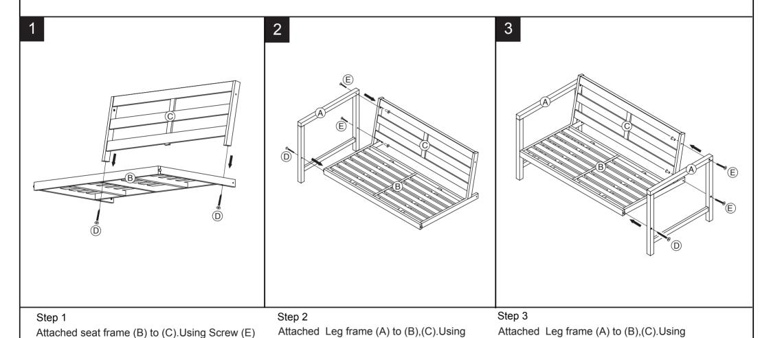
Screw(D) tighten by (F), and Bolt (E)
