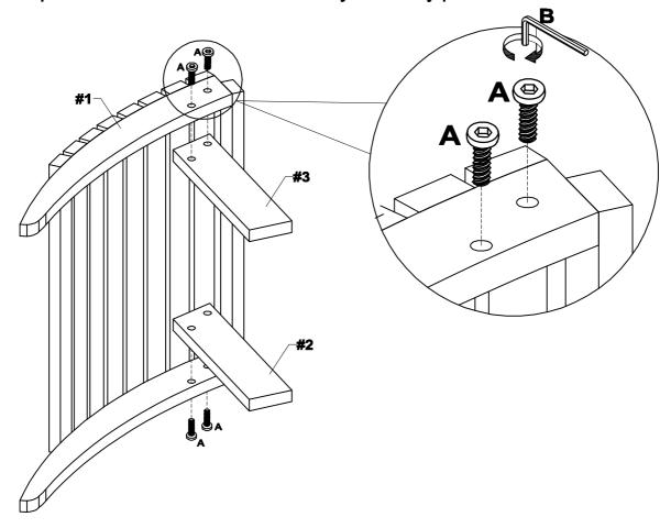
IMPORTANT: DO NOT TIGHTEN BOLTS COMPLETELY UNTIL ALL BOLTS ARE COMPLETELY LINED UP AND INSERTED INTO HOLES.
