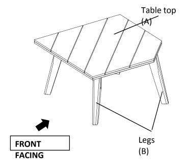
This Table has multiple parts and may require up to 30 minutes to assemble. To give you an overview of the Table parts, the above picture is to help you put the various parts into perspective. Please read through the instructions below to familiarise yourself with the parts and steps before assembly.
