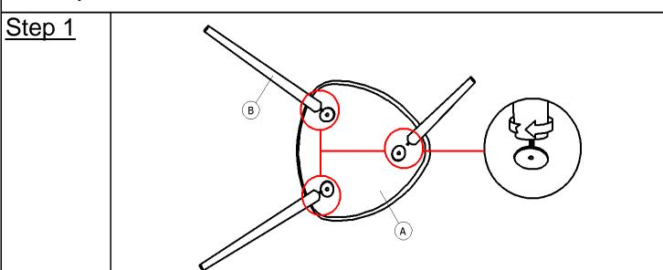
Open the carton and place all parts onto a clean, non-marring surface. Insert **one of** Leg(B) into the base of the Table Top(A) as shown above and tighten by turning the Leg clockwise by hand.
