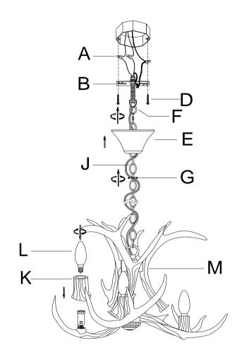
Insert the bulbs(L) into the sockets until secure. **DO NOT EXCEED THE SPECIFIED WATTAGE.**
