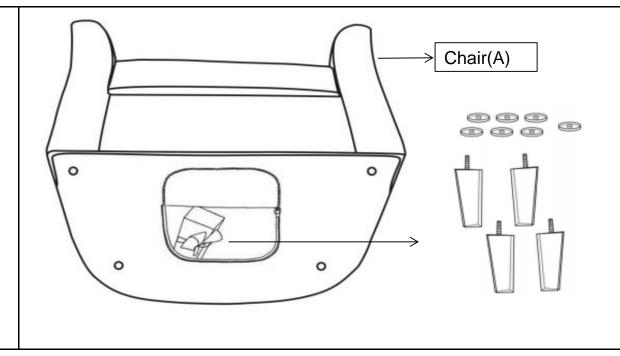
Position the Chair on its back, as shown. Unzip to open and remove the 4 wooden legs. Close the Poket.
