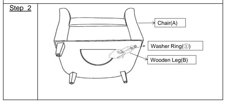
Install Wooden Leg(B) into the Chair by putting a Washer Ring(1) on the threaded stem and then insert the threaded stem into the threaded hole at each corner of the bottom of the Chair.
