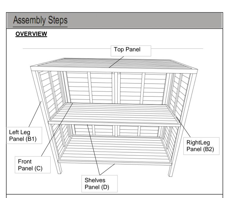
This Bar Table has multiple parts and may require up to 30 minutes to assemble. To give you an overview of the Bar Table parts, the above picture is to help you put the various parts into perspective. Please read through the instructions below to familiarise youself with the parts and steps before assembly.
