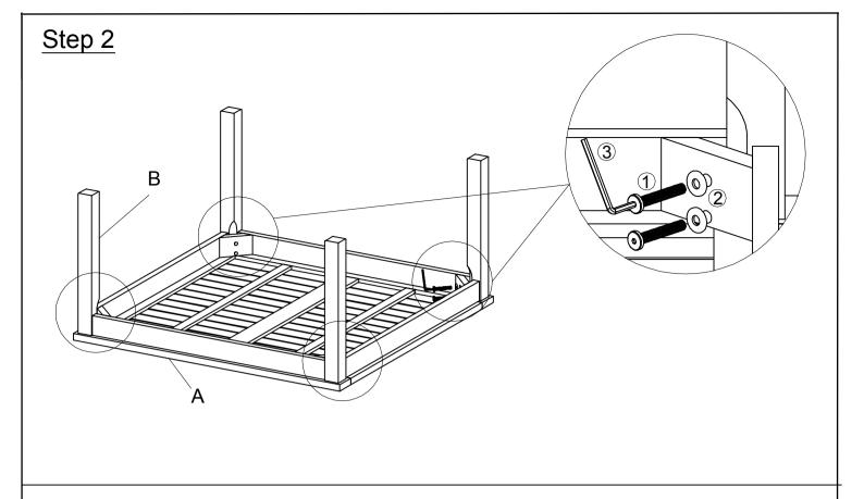
Attach Leg(B) to the Table Top(A) using Bolt (1) and Washer(2) with Allen Key(3). **Do not fully tighten the Bolts.**
