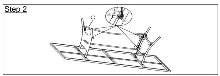
Attach Leg Support Panel(C) between Leg Panels(B) using Bolt(2) and Washer(3) with Allen Key(1) as shown in the picture above.
