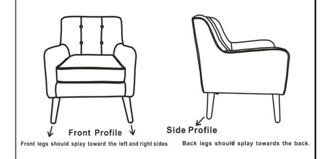
Make sure all the parts are connected and securely locked into position and Legs are in the correct positions.
