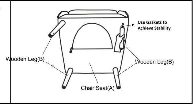
Install the Wooden Leg(B) into the Chair Seat(A) by putting a Gasket(1) on the threaded stem of the Leg.
