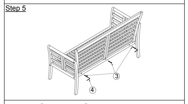
Use Short Screw  $(\mathfrak{T})$  and Allen Wrench  $(\mathfrak{T})$  to attach Backrest Panel (A) and Seat Panel (D).
