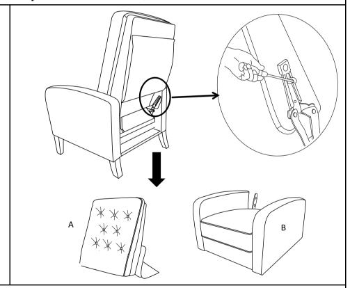
Disassembly Note:Open the flap on the Chair Backrest(A),use a screwdriver (Don't use fingers) pressing outward on the metal ear on the pre-attached Metal Bracket on one side of the Chair Backrest(B). With assistance of you adult partner to keep the Chair Base(B) in place, pull out the Chair Backrest(A) upward at the same time,repeat the same step for another side.
