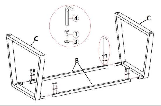
Carefully place the Leg Frame(C) and Support Rail (B) on a clean, non-marring surface as picture, align the mounting positions on Leg Frame(C) with the mounting positions on Support Rail (B), then attach them together by using Washers(③) and Short Bolts (①) with Allen Key (④).
