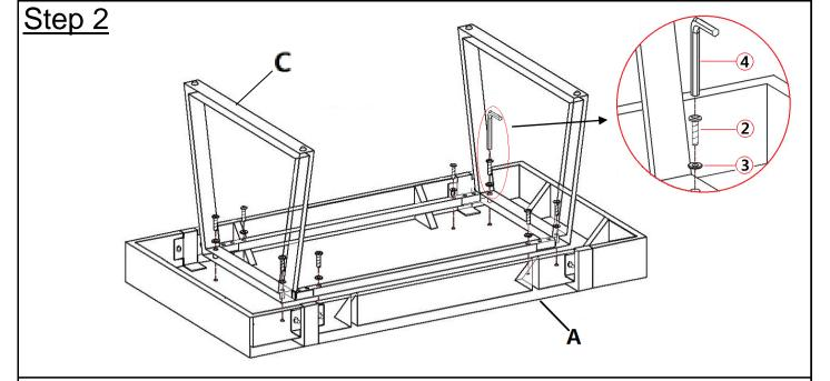
Carefully place the Table Top (A) facedown on a clean, non-marring surface with assistant from second adult. Align the mounting positions on assembled Leg Frame(C) and Support Rail (B) with the mounting positions on Table Top (A), then attach them together by using Washers(③) and Long Bolts (②) with Allen Key (④).
