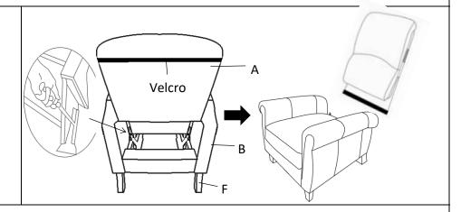
Disassembly Note:open the flap on the Ghair Backrest(A),use a screwdriver(Don't use fingers) pressing outward on the metal ear on the preattached Metal Bracket on one side of the Chair Base(B),with assistance of you adult partner to keep the Chair Base(B) in place,pull out the Chair Backrest(A) upward at the same time,repeat the same step for another side. Then the Chair Backrest(A) can be taken out.
