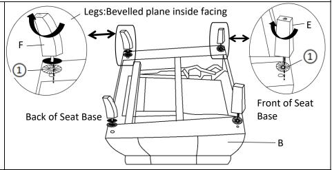
Keep the Chair Base with Footrest(B) in the same position. First, install the Front Legs(E) at the bottom of the Chair by placing one Gasket① on the threaded stem.
