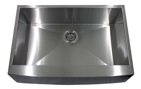
This Pro Series Apron gives a conteporary spin to the traditional farmhouse sink. The bottom of the sink has channel grooves to divert water for proper drainage. Crafted from 304 16 gauge Stainless Steel with a satin finish. Nantucket Sinks are sprayed with a special insulation to reduce condensation. Rubber padding is applied for noise reduction.
