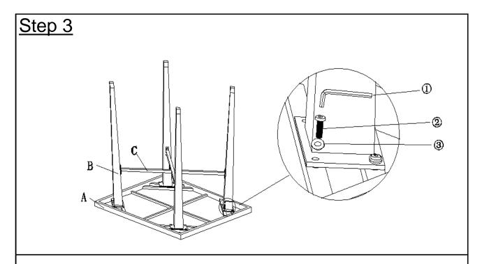
Finally attach Legs(B) to Table Top(A) using Bolts(2) and Washers(3) with Allen Key(1) at the inside mounting positions.
