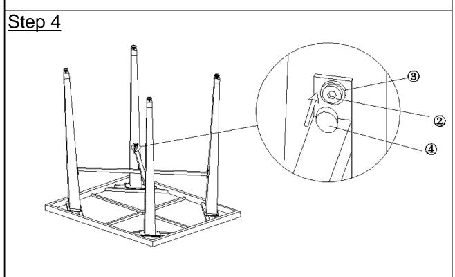
Now fully tighten all Bolts at all joints in a sequential manner.
