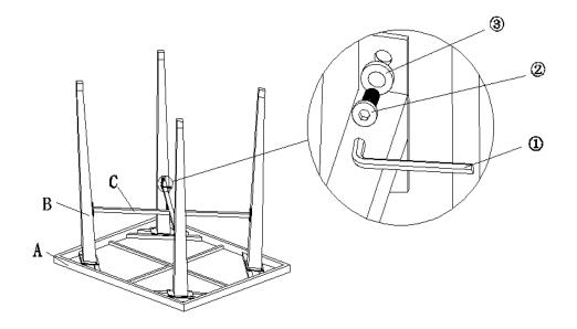
Attach Connector(C) between Legs(B) using Bolts(2) and Washers(3) with Allen Key(1) as pictured.
