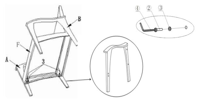
Put the Love Seat(F) against the Left Armrest(A) and line up the three mounting positions of both. Attach the Love Seat(F) to the Left Armrest(A) using Bolts(2) and Washers(3) with Allen Key(4). **Only loosely tighten Bolts.**
