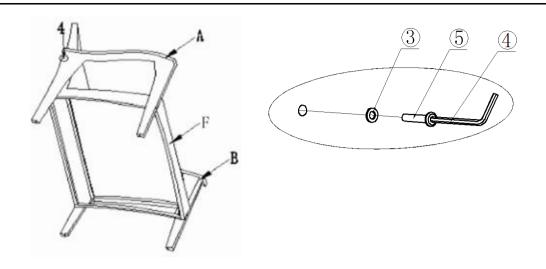
Turn the Love Seat over, and attach Bolt(5) and Washer(3) using Allen Key(4) as pictured above. **Only loosely tighten Bolts.**
