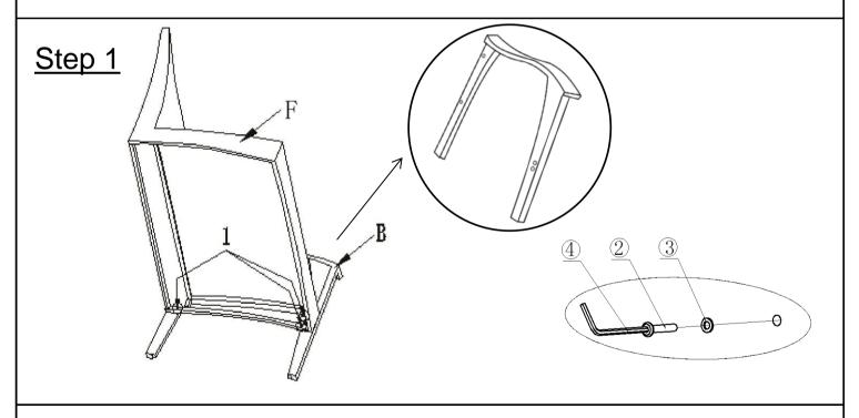
Open the carton and place all the parts onto a clean, non-marring surface. Put the Love Seat(F) against the Right Armrest(B) and line up the three mounting positions of both. Attach the Love Seat(F) to the Right Armrest(B) using Bolts(②) and Washers(③) with Allen Key(④). Only loosely tighten Bolts.
