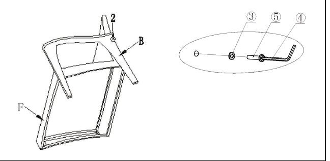
Turn the Love Seat over, and attach Bolt( $\mathfrak{S}$ ) and Washer( $\mathfrak{S}$ ) using Allen Key( $\mathfrak{S}$ ) as pictured above. Only loosely tighten Bolts.
