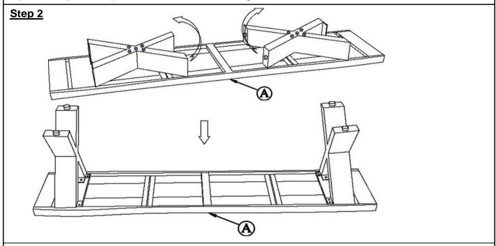
Place the Bench (A) facedown, onto a clean, soft surface to avoid any scratches or damages to the product.
