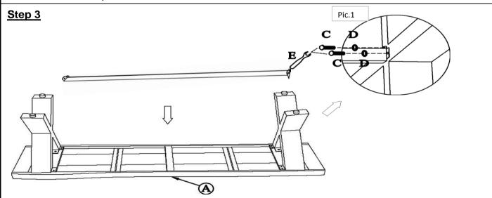
Attach the Support Bar (B) to the Bench (A)
