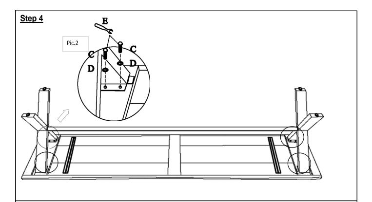
Secure Legs to Bench by using Bolts (C) and Flat Washers (D) with Spanner Wrench(E) as shown in Pic.2 at all 8 positions.
