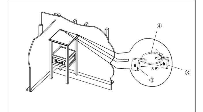
**C**: Move the Cabinet against the wall. Then pull the Cabinet Restraint Strap(4) through two Metal Brackets(3) one by one, lock tight the Cabinet Restraint Strap(4), as shown above.
