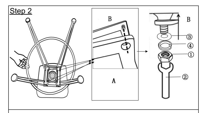
Place the Seat(A) facedown, then align the Leg Frame(B). Attach the Leg Frame(B) to Seat(A) using Nuts(1), Spring Washers(4) and Washers(3) with Spanner(2).
