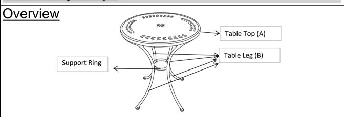
This Table has multiple parts and may require up to some 20 minutes to assemble. To give you an overview of the Table parts, the above picture is to help you put the various parts into perspective. Please read through the instructions herebelow to familiarise the parts and steps before assembly.
