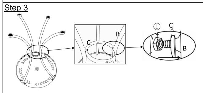
Attach the Support Ring(C) to Table Legs(B) using Nuts( $\bigcirc$ ) with Spanner( $\bigcirc$ ). Loosely tighten Nuts.
