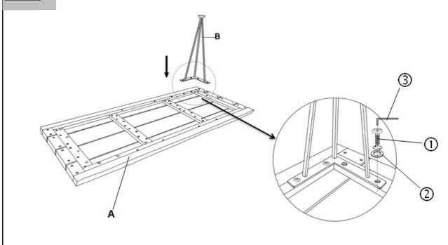
Insert leg (B) into the table top  $\,$  (A), put the flat washers (  $\,$  (2 ) and bolt (1) as above picture.
