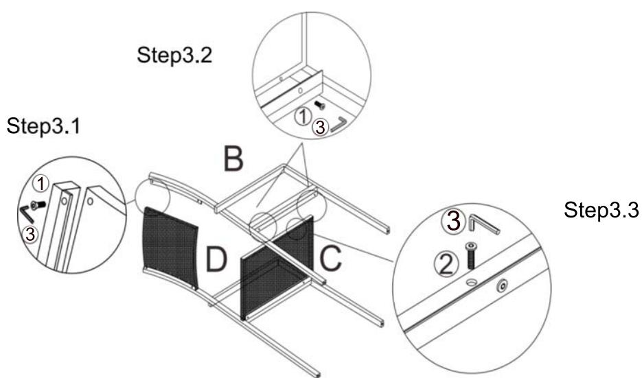
**3.1)** Attach the Left Armrest/Leg(B) to Backrest(D) using Bolts(①) with Allen Key(③) as shown above.
