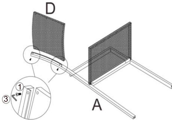
Attach Backrest(D) to Right Armrest/Leg(A) using Bolts(①) with Allen Key(③) as shown above.
