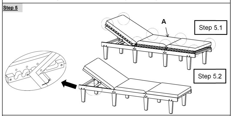
Stand the Lounger right side up onto a flat horizontal surface and adjust to achieve levelness. Inspect it and make sure all parts are adequately connected.
