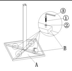
Attach the Table Top (A) to the Mounting Cross (B) and Table Leg (C) using Bolt (1) Washer(2) with Allen Key (3) as shown in Picture.
