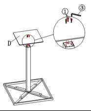
Attach the Base panel (D) between the Table Leg (C) using Bolt (1) with Allen Key (3) as shown in Picture.
