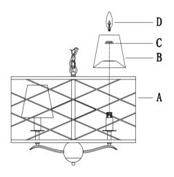
PLEASE USE ON/OFF TYPE"B" BULB MAX 40-WATT OR CFL BULB MAX 9-WATT THERE ARE 6PCS 25-WATT TYPE "B" BULB IN THE BOX
