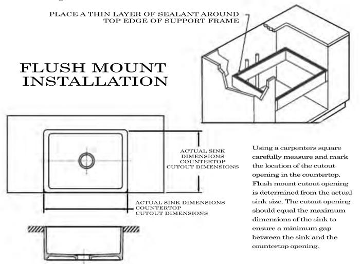
Note: Check dimensions as a reference and measure the sink being installed.
