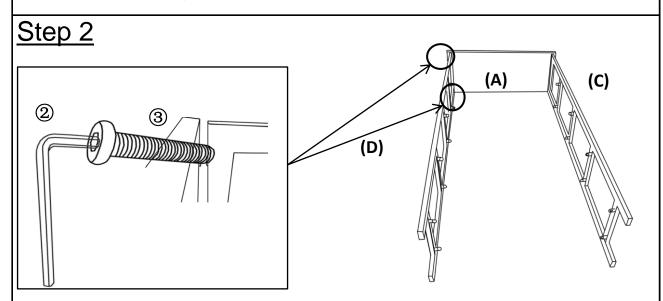
Attach Right Frame(D), with pre-attached nut is upwards, using Bolts(2) with Allen Key(3).
