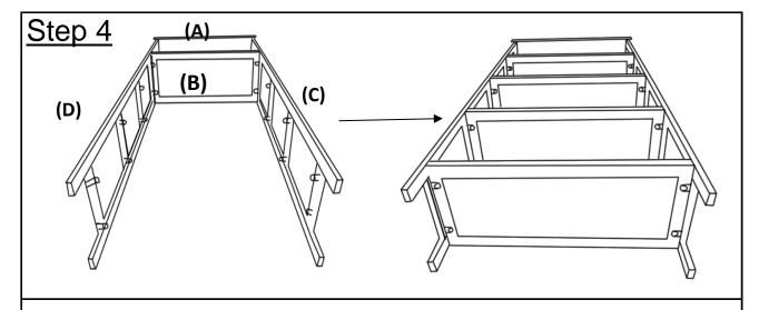
Repeat the process from Step 3 to attach the remaining Wooden Shelves. **Only loosely tighten the Bolts.**
