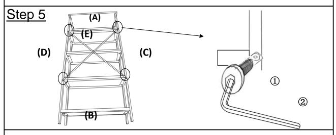
Rotate the "X" Iron Stretcher(E) to the required position as shown. Attach "X" Iron Stretcher(E) to the Bookcase(E) using Bolt(1) with Allen Key(2). Remind: This "X"Iron Stretcher (E) is packed on beside of Left Frame (C).
