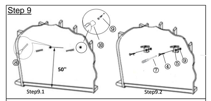
9.1) Use Power Drill((a)) Drill two mounting positions on wall at same height, bury Plastic Anchor((9)) into the mounting position with a hammer((10))(Not priovide).
