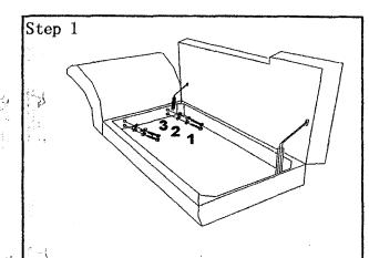
Assemble back (C) to Seat frame (A) by using bolt (1), spring washer (2) and washer (3) as shown.
