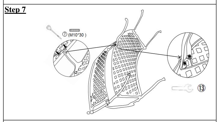
Lock two M10\*30mm Bolts( $\bigcirc$ ) to the underside of the Seat Panel(B) by using the Screwdriver( $\bigcirc$ 1).
