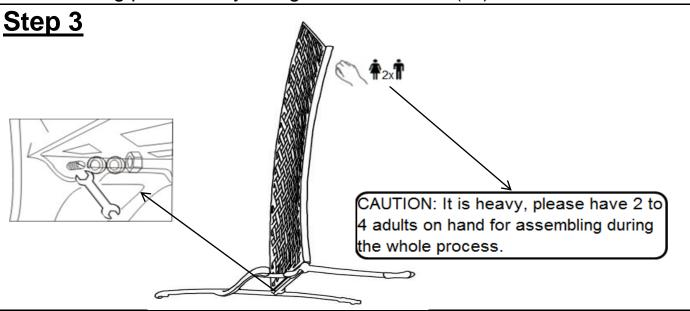
Hold the Seat Panel(B) up and align the mounting positions to the Bolts(③) on the Left Armrest(C).
