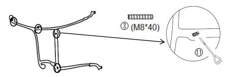
Place the Left Armrest(C) on the floor and lock four M8\*35mm Bolts(③) to the mounting positions by using the Screwdriver(①).
