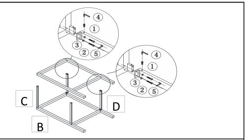
Attach Leg(B) to Top Side Bars(C) and Footrests(D) using Bolts(2) and Washers(3) with Allen Allen Key(5) as shown above.
