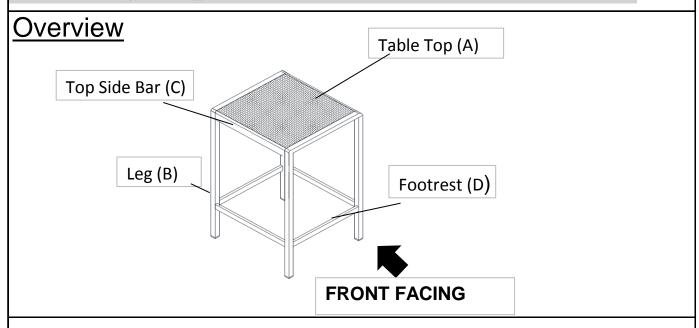
This Table has multiple parts and may require up to 30 minutes to assemble. To give you an overview of the Table parts, the above picture is to help you put the various parts into perspective. Please read through the instructions below to familiarise yourself with the parts and steps before assembly.
