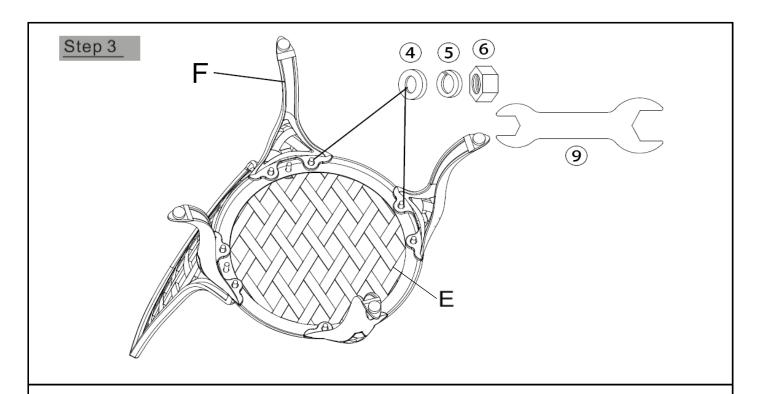
Insert the Legs(F) onto the Bolts on the Chair Seat(E).
