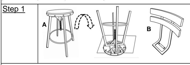
Put the parts on a clean, non-marring surface. Place the Seat (A) facedown onto a table, as shown.
