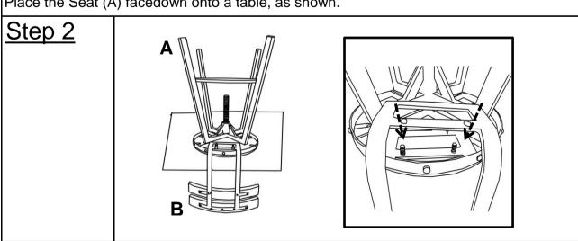
Align the mounting positions on the Seat(A) and the Backrest(B).
