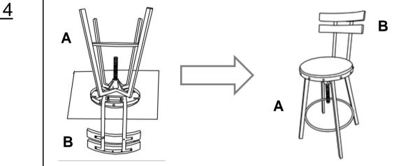
Stand the Barstool up and check the firmness of backrest, tighten all nuts.
