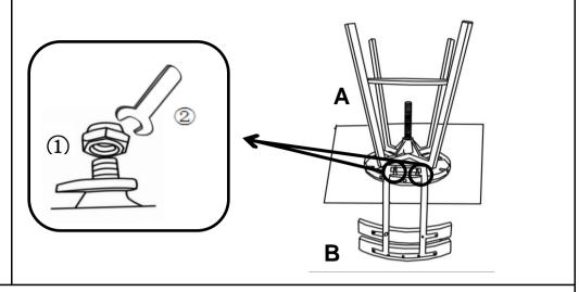
Attach Seat (A) to Backrest(B) using Nuts(1) with Wrench(2). CAUTION: When tightening these Nuts, tighten sequentially. DO NOT tighten any screw fully and then towards the next one.
