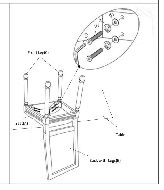
Place the Seat(A) on the side of a table, with the Backrest facing down and perpendicular to the Desk Top, as pictured. Insert Front Legs(C) into the mounting positions of Seat(A) and attach using Bolts(1), Spring Washers(2), and Washers(3) with Allen Key(4).
