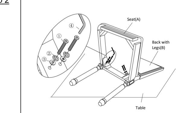
Place the Back with Legs(B) on a clean, non-marring surface. Align the mounting positions of the Seat(A) and Back with Legs(B), then attach them using Bolts(1), Spring Washers(2) and Washers(3) with Allen Key(4).
