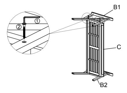
With assistance from your adult partners, turn the Chair into the other side Repeat the same process of step 2 to secure Left Leg Panel (B1) with Seat Panel (C) by using Screw (2) and Allen Wrench (1)
